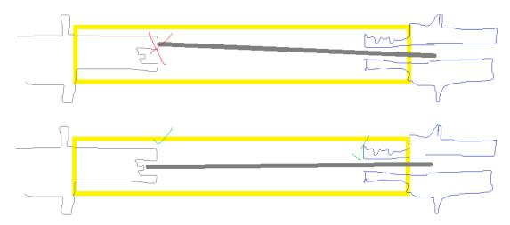
You can bring it in the position like shown on the lower picture by shacking the unit by hand and fasten the rod-ends carefully. Otherwise you will push up the upper valve core and this might damage it.
