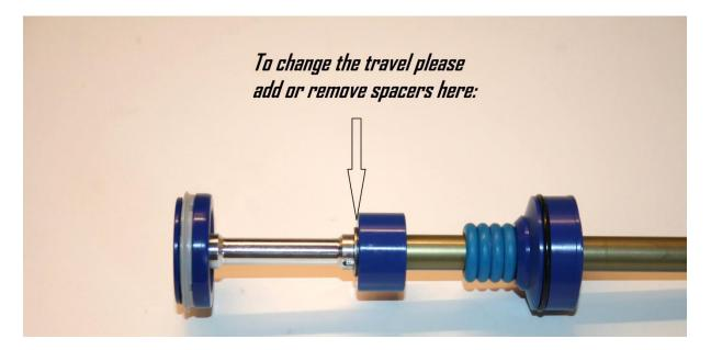
For this you have to take a 9mm and 11mm wrench. Disassemble one of the ends (doesn't matter which one) and you can swap the spacers.
