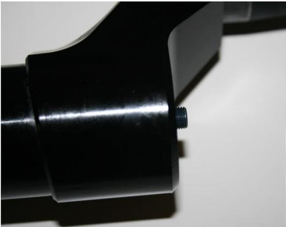
Push the lower to the top until you can see the valve / damping end.
