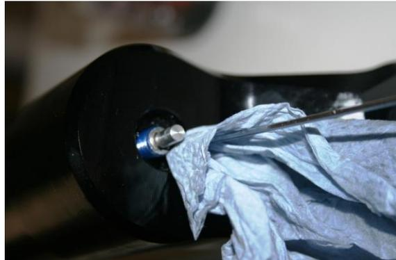
Unscrew the hex nut with a 10mm socket nut. Afterwards pull out the lower tube carefully and release the old oil out of the upper leg. And clean the inside.
