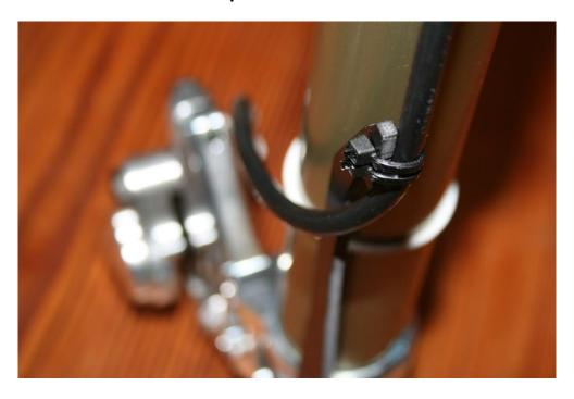
The brake cable has to come from the inside to avoid contact between the cable and the upper leg in case of compression.
