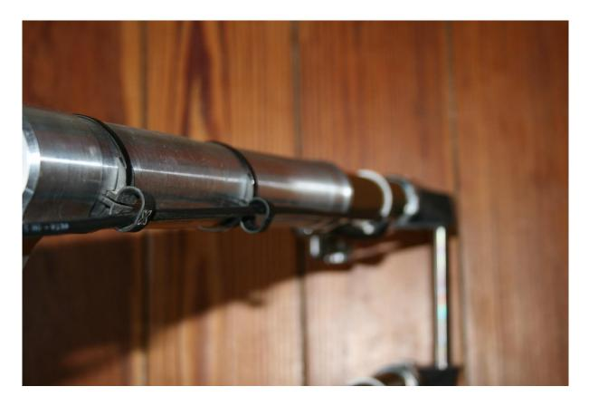
Then install the upper guides as usual. The lower one has to have a minimum distance to the hose arm bigger than the fork stroke to avoid contact in case of compression.
