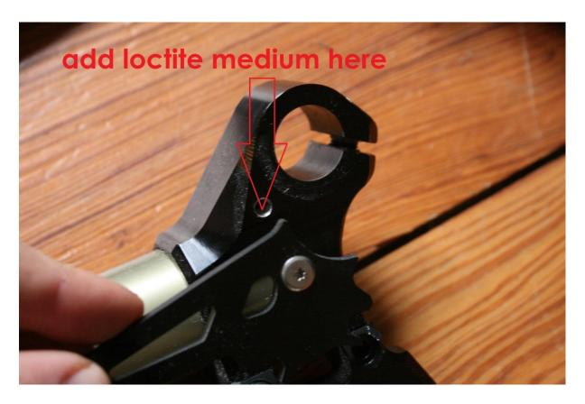
Then mount the hose guide arm with the bolt. TX10 – around 3-4 Nm.
