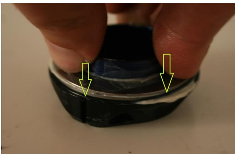
Then put the O-ring onto the bearings in the groove. Make sure that it does not lay between the bearing washers. For this it might be necessary to put some pressure on the waser with 3 fingers.
