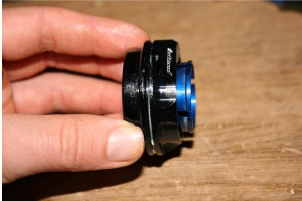
Push the lower cup with the already pressed in radial bearing onto the unit. By pushing all together, the blue shell comes out through the upper cup with. Ensure a proper and smooth run of the unit. If not, maybe the o-ring is anywhere where he shouldn't be. If you put in everything correctly, you will feel a smooth run of the headset in the assembly step shown on the right side.
