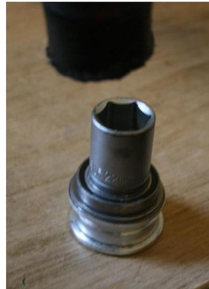
If so, disassemble the unit and a press out the inner shell with a **22mm** (smaller than 30mm) nut to push out the inner shell like shown in the picture. You need any underlayment with an inner diameter of > 32mm to be able to push out the inner shell.
