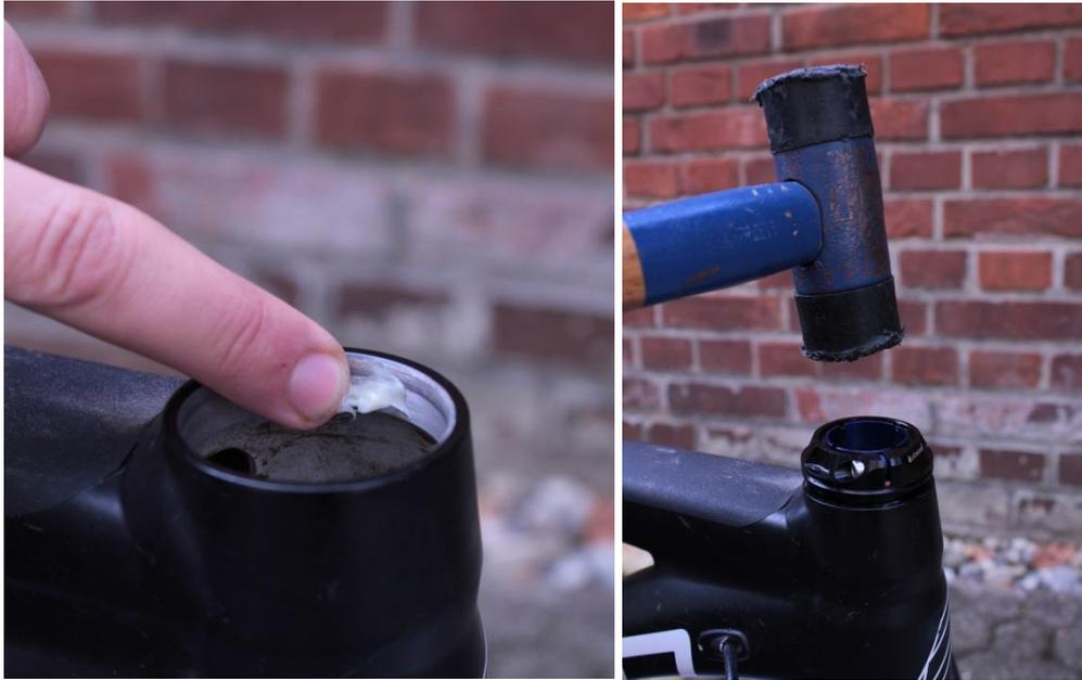
Put Spacers, stem and headset on the steerer tube and preload the headset (as tight as possible without influencing a smooth run)
