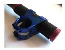
After assembly of the stem and fastening of the bolts please check if the stem is really fixed on the steerer by clamp the front wheel between your legs an try to turn the handlebar.
