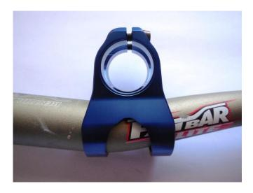
To get the handlebar in the stem the handlebar clamp has to be opened slightly with the included wooden spoon. The easiest way is shown in the pic, look at the chamfer! (Fase am Holz)! Please note that the wooden spoon should not extend in the handlebardiameter because the handlebar should take place there later.
